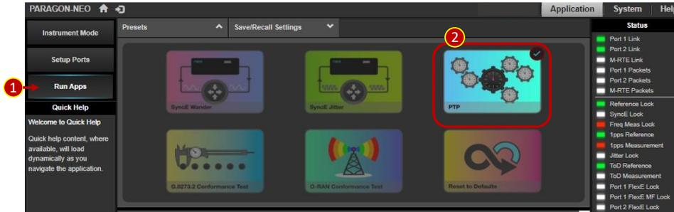
3. In the **PTP Emulation** section of the GUI, set **Test Mode** = **M-Clock** and select a **PTP Profile** from the drop-down list to match the PTP profile that the PRTC + T-GM runs.
