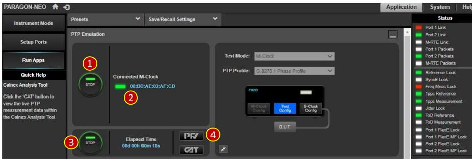
5. In the PFV browser window, check that the PTP profile used by the PRTC + T-GM conforms to the required PTP Profile.
