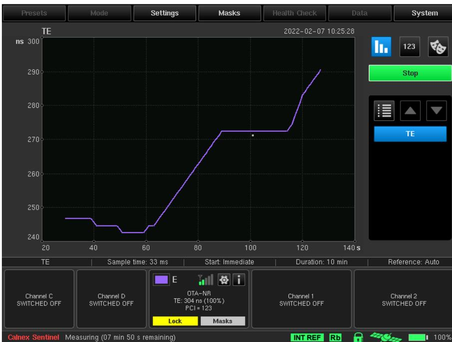
In this case Sentinel will initiate a new search to try and find the signal again before continuing the measurement. When successful, the lock LED will turn yellow to indicate that lock was lost during the measurement. It will turn green again when the measurement is completed.
