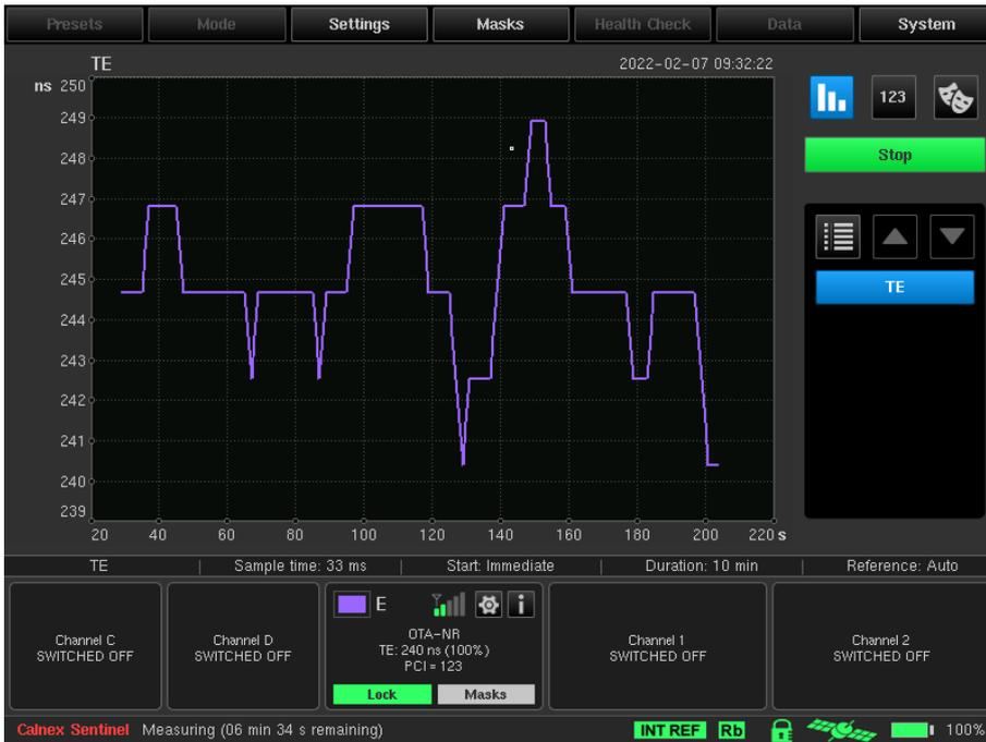
If Sentinel fails to make a sufficient number of successful measurements within a particular time window, then the measurement is deemed to have gone out of lock – this will be indicated by a red Lock LED.
