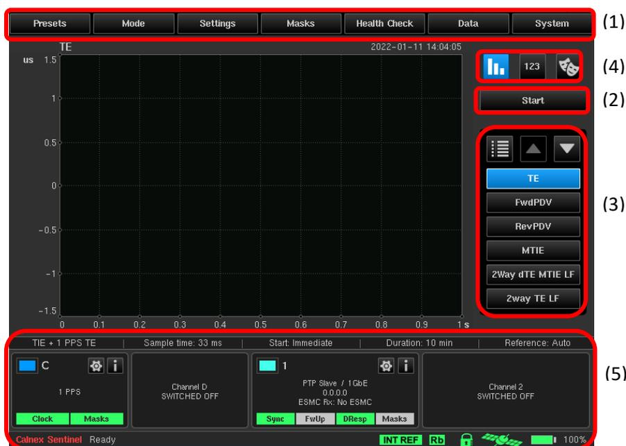
The main screen contains controls to allow simple, ordered configuration (1) and operation (2) of Sentinel. Navigation buttons allow movement between each measurement result graph (3) and change the mode of viewing results (4). The status of the measurement sub system is shown in widgets and icons at the bottom of the screen (5).
