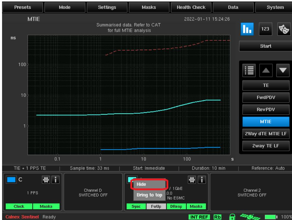
The MTIE of PTP is shown on the **2way dTE MTIE LF** graph along with the ITU-T G.8271.1 network limits mask. The signal passes if the 2way MTIE values remain below the line.
