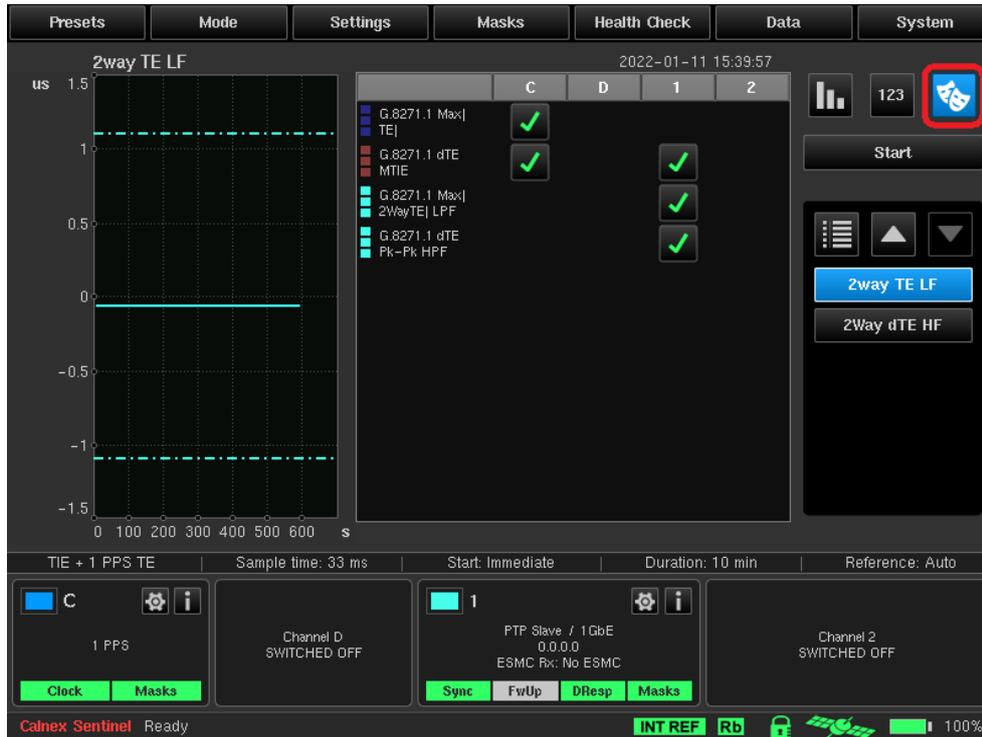
Each populated measurement channel has an associated widget to indicate the status and configuration of the channel and to allow quick access to the channel settings.
