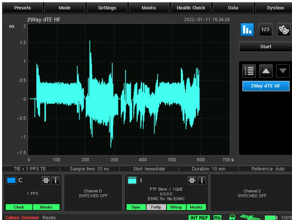
The PTP message statistics for the measurement duration can be viewed by adding the **PTP Statistics** metric from the **Graph Selection** screen.
