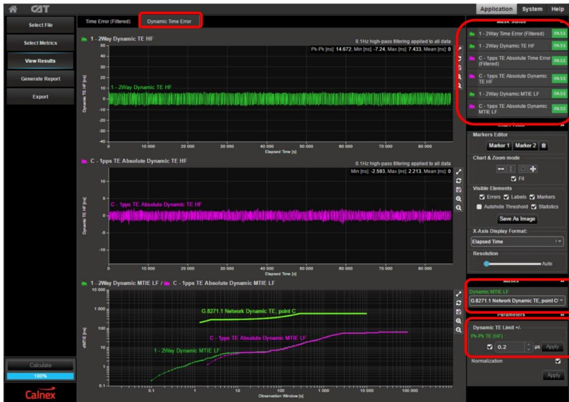
Select the **G.8271.1 Network Dynamic TE, point C** mask under Dynamic MTIE LF in the lower right of the display and set the Dynamic TE Limit +/- to **0.2µs**, tick the box and select **Apply**. Press the **Calculate** button at the lower left of the screen and wait for the status bar to reach 100%.
