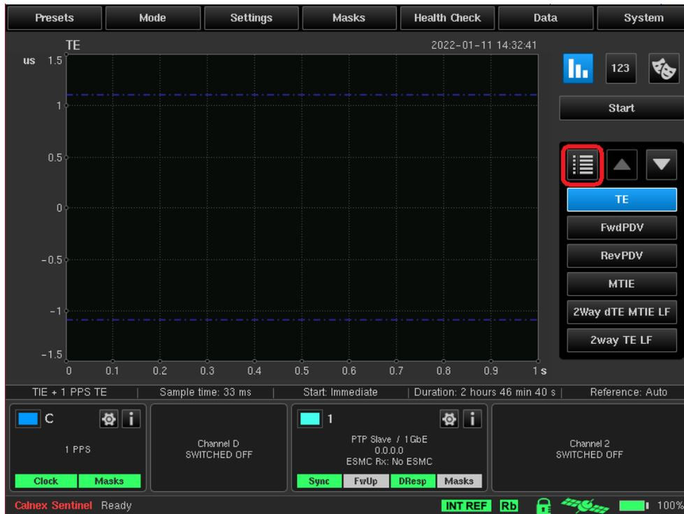
A **Hide/Show** checkbox and associated measurement description is available for each graph. Graph ordering can be changed by highlighting the graph name and pressing the **Order** arrow buttons.
